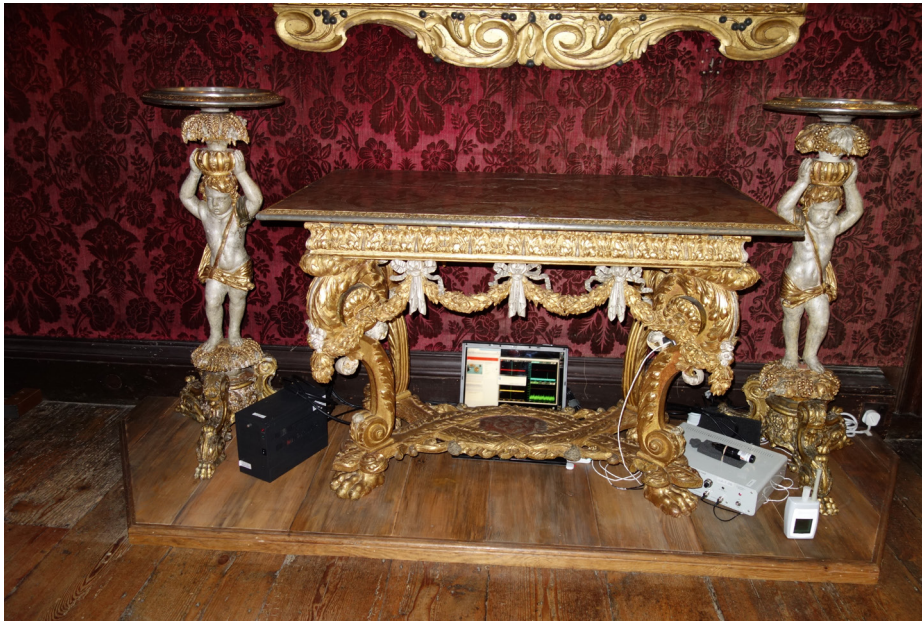
Fig. 5 Gole Suite table and torchère in Cartoon Gallery with AE monitoring equipment. AE sensors connect to the amplifier (right), which is linked by the PCI interface (left) to the laptop (rear centre). Hanwell T and RH sensor temporarily located in the foreground. (© National Trust)
