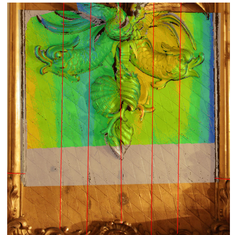
Fig. 7 Combined illustration of photography and assessment of the structured light scanner (March-October 2015). The red lines mark the joints.
