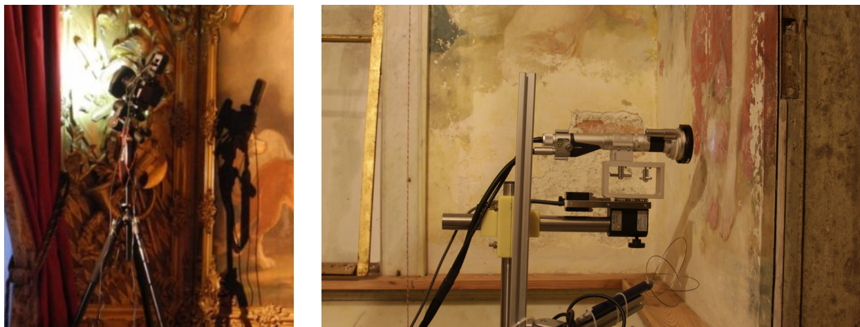
Fig. 4 Left: time-lapse pictures with a SLR-camera in the eastern tapestry room. Right: 3D-microscopy of the wall paintings in the bathroom. (Source: BSV)
