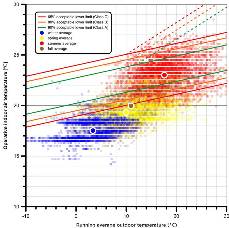
Fig. 4 Collected indoor temperatures measured in 2009, 2010, 2013, 2014, 2015 and 2016 in the Salon as a function of outdoor temperatures. The comfort limits for an “alpha” building in which the user has limited control over the indoor temperature by e.g. opening windows, is presented using the so-called Adaptive Thermal Model, extracted from Van der Linden et al [2006].
